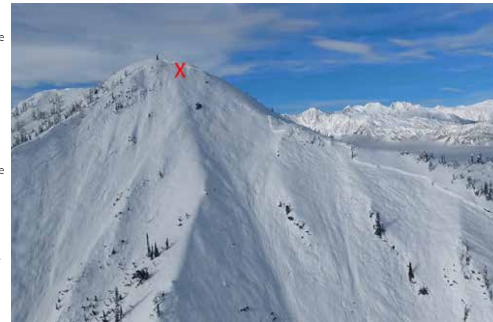
FIG. 3: START ZONE DETAIL OF JACK MACDONALD. THE RED "X" MARKS THE 13 KG ANFO SHOT LOCATION. ROUGHLY HALF THE ENTIRE CROWN WIDTH IS DEPICTED.
