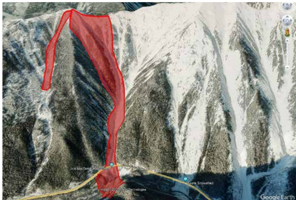
FIG. 5: A GOOGLE EARTH IMAGE SHOWING THE WRAPAROUND SIZE THREE AVALANCHE IN HELEN'S TO THE LEFT OF THE MAIN AVALANCHE IN JACK MACDONALD. THE CROWN IN JACK MACDONALD PROPAGATED ACROSS ROUGHLY ONE-THIRD OF THE START ZONE AND INVOLVED THREE MAJOR GULLY SYSTEMS. THE SYMPATHETIC SIZE 3.5 ON THE NORTH ASPECT THAT RAN ALL THE WAY TO THE TANGIER RIVER IS NOT SHOWN.
