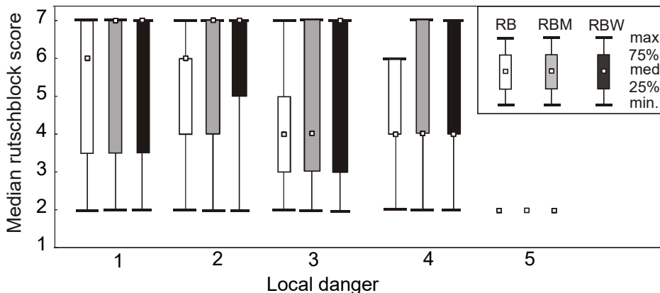
Figure 3. Rutschblock variables RB, RBW and RBM for each level of local avalanche danger.
