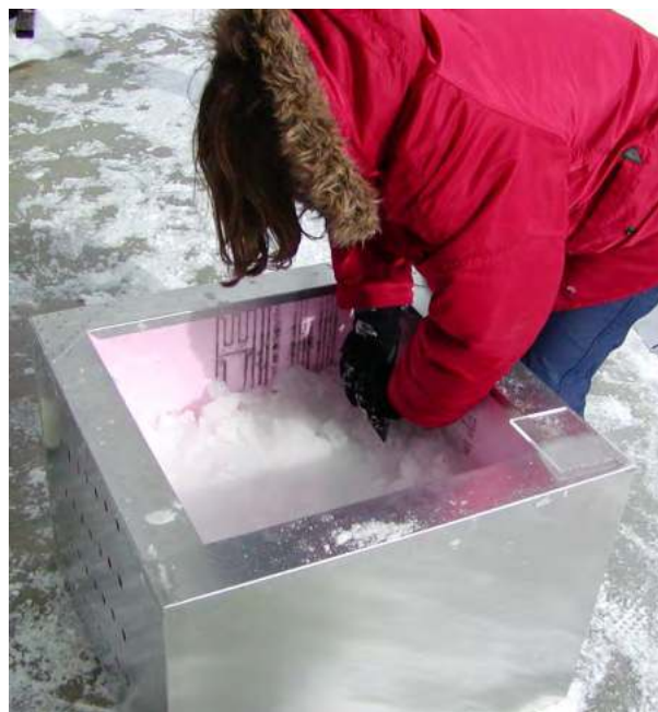
Figure 3. Spreading wet snow layer evenly onto dry snow base.
