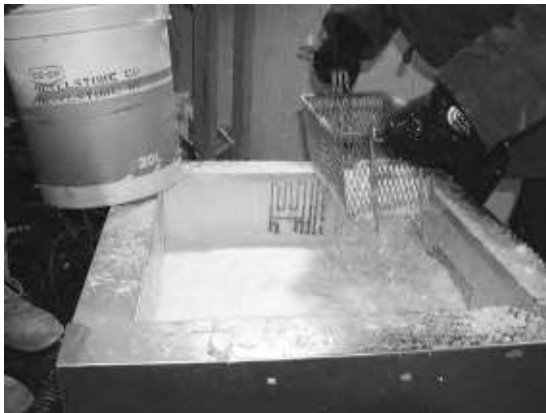
Figure 4. Sieving fresh snow onto the wet layer.
