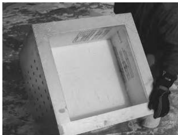
Figure 2. Laterally insulated box with base snow layer. The side of the box at the bottom of the photo is removable to facilitate crystal extraction.
