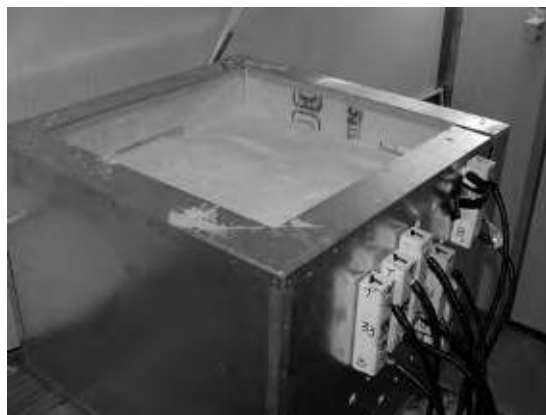
Figure 5. Laterally insulated box with thermistors placed to monitor temperature in air and in three-layer snow specimen.
