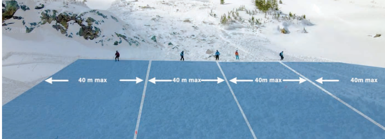
THE LANE (OR SEARCH STRIP WIDTH) FOR EACH SEARCHER IS DEPENDENT ON THE SCENARIO BUT CAN VARY FROM AS NARROW AS FIVE METRES TO AS WIDE AS 40 METRES, OR EACH MANUFACTURER'S MAXIMUM RECOMMENDED SEARCH STRIP WIDTH.
