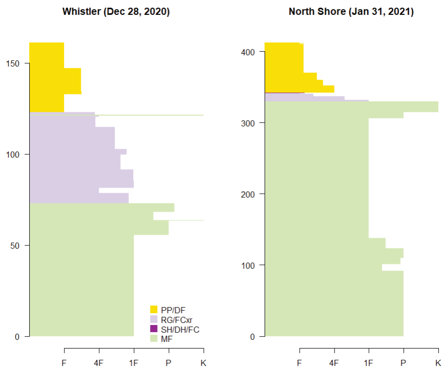
FIG. 2: THE SIMULATED SNOW PROFILE FROM WHISTLER ON DEC 28, 2020 (LEFT) IS MISSING THE PERSISTENT WEAK LAYER BENEATH THE NEW SNOW THAT RESULTED IN MANY AVALANCHE ACCIDENTS, WHILE THE PROFILE FROM THE NORTH SHORE ON JAN 31, 2021 CLEARLY SHOWS THE WEAK LAYER ABOVE A CRUST THAT ALSO RESULTED IN ACCIDENTS.
