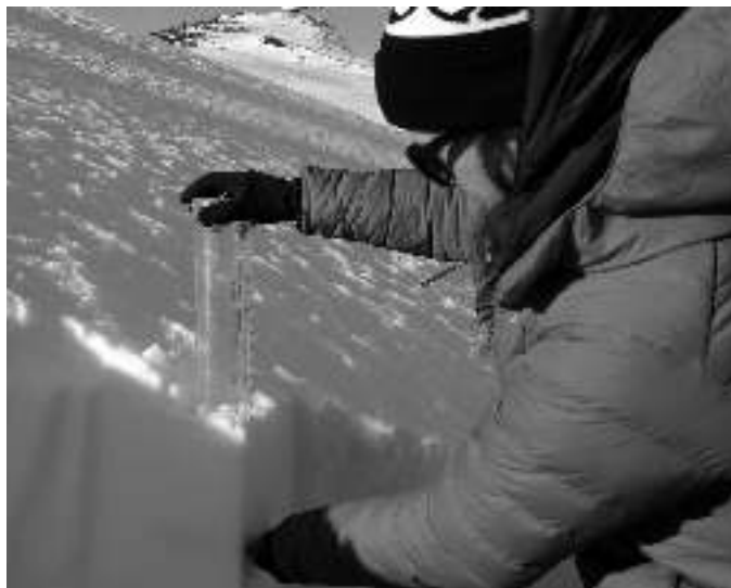
INSTRUCTORS WILL BE DEMONSTRATING HOW DENSITY IS MEASURED IN THE FIELD AND SPEND MORE TIME EMPHASIZING THE IMPORTANCE OF DETERMINING WATER EQUIVALENCY. PHOTOS: STEVE CONGER
