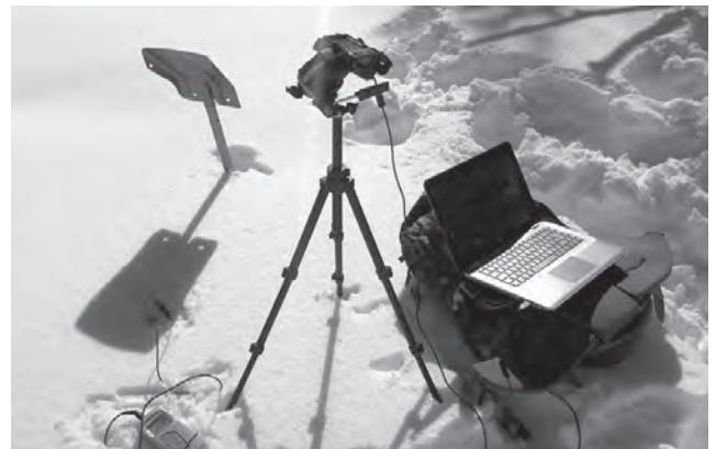
FIG. 6: EXPERIMENT IN 2014 TO COMPARE THE READINGS FROM TWO CONTACT THERMOMETERS IN THE SHADE OF THE SHOVEL AND AN IR THERMOMETER (NOT SHOWN).
