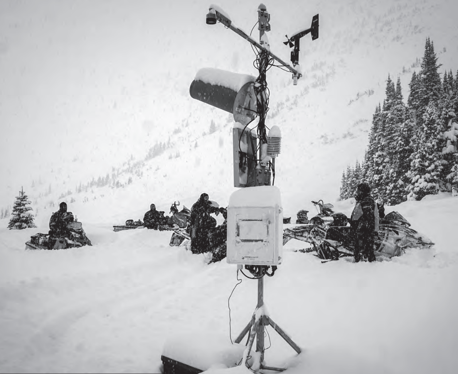
INSTALLING A WEATHER STATION IN THE KAKWA WILDERNESS AREA, WITH THE HELP OF THE SWAN CITY SNOWMOBILE CLUB OUT OF GRANDE PRAIRIE, AB //RYAN BUHLER
