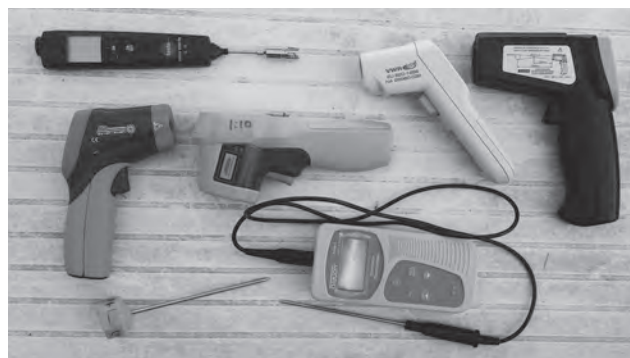
FIG. 3: CONTACT THERMOMETERS (BIOS IN BOTTOM LEFT, OAKTON ACORN IN BOTTOM RIGHT) AND FIVE IR THERMOMETERS (ABOVE), FOUR OF WHICH ARE PISTOL-SHAPED.
