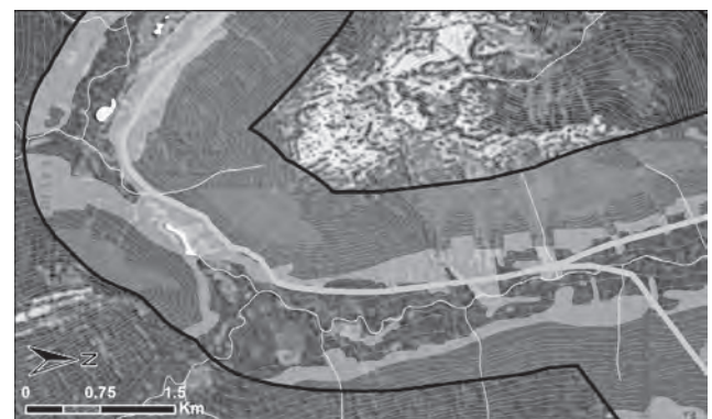
FIG. 5: EXAMPLE OF ATEs ZONE MAPPING (TBL. 2) FOR AN ENERGY CORRIDOR. ATEs CLASSES ARE INDICATED BY COLOUR (CLASS 1, (CLASS 2), (CLASS 3), (CLASS 0) (CAMPBELL AND GOULD, 2014).
