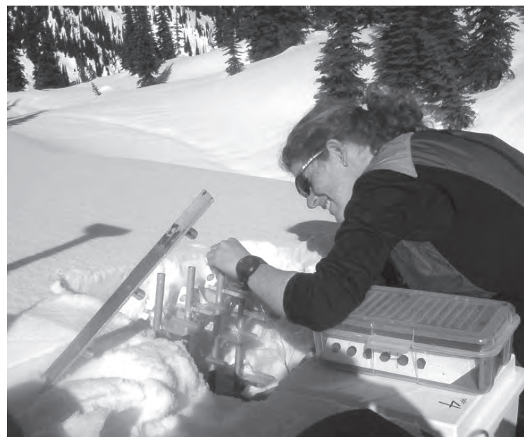
LAURA BAKERMANS USING A JIG TO PRECISELY PLACE THERMISTORS NEAR THE SNOW SURFACE // ASARC
