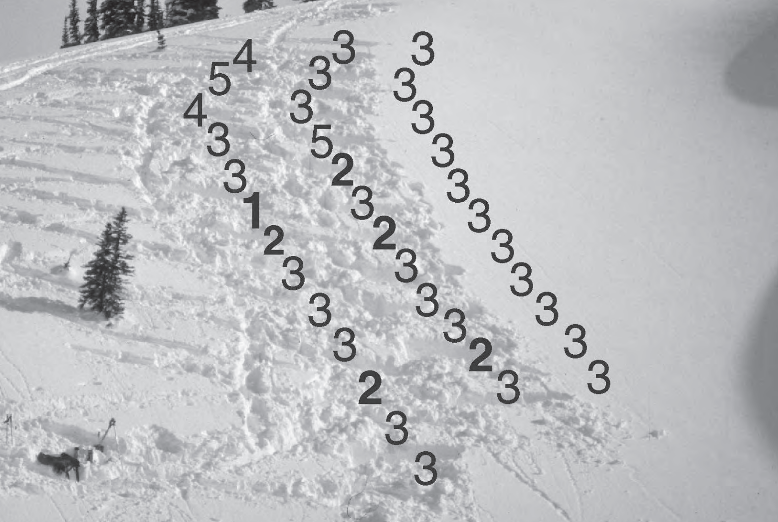
AN ARRAY OF RUTSCHBLOCK TESTS ON A WEAK LAYER OF SURFACE HOAR FROM 1991. MARK SHUBIN AND BRUCE MADE THE THIRD ROW OF TESTS AFTER THE PHOTO WAS TAKEN. NOTE THAT A SINGLE TEST IN THE TOP LEFT PART OF THE ARRAY GIVES A MISLEADING INDICATION ABOUT LOCAL STABILITY // BRUCE JAMIESON
