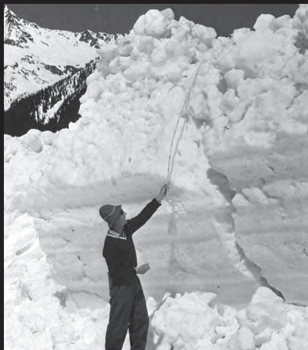
PETER SCHAEERER MEASURING THE DEPTH OF A WET SNOW AVALANCHE DEPOSIT AT MACDONALD WEST NO. 4 SLIDEPATH. MAY 4, 1957
