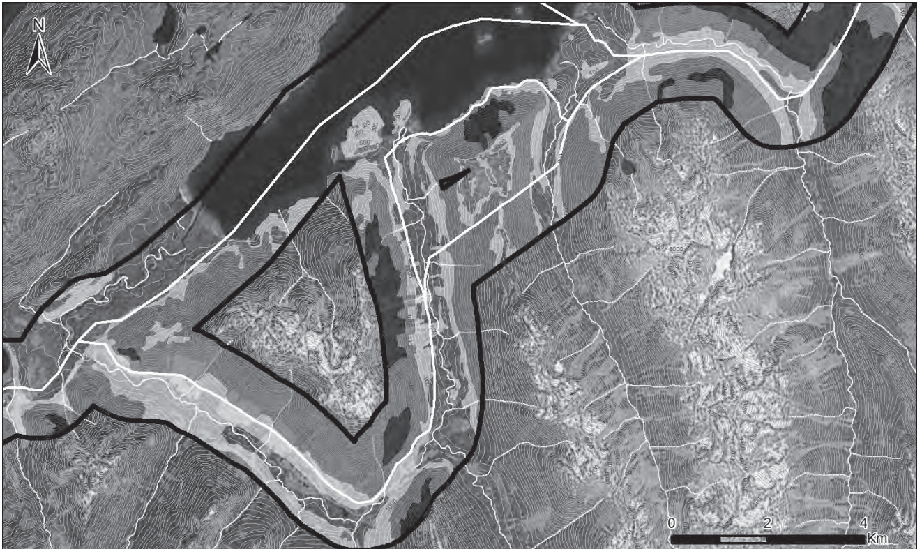
FIG 1: EXAMPLE OF ATES ZONE MAPPING FOR AN ENERGY CORRIDOR (WHITE LINE). ATES CLASSES ARE INDICATED BY SHADING WITH LIGHT GREY AS CLASS 1, DARKER GREY AS CLASS 2, DARKEST GREY AS CLASS 3, AND NO SHADING WITHIN THE STUDY AREA (BLACK OUTLINE) AS CLASS 0. PLEASE NOTE: GREEN-BLUE-RED COLOURED ATES ZONES WERE CONVERTED TO GREYSCALE FOR THIS PUBLICATION.
