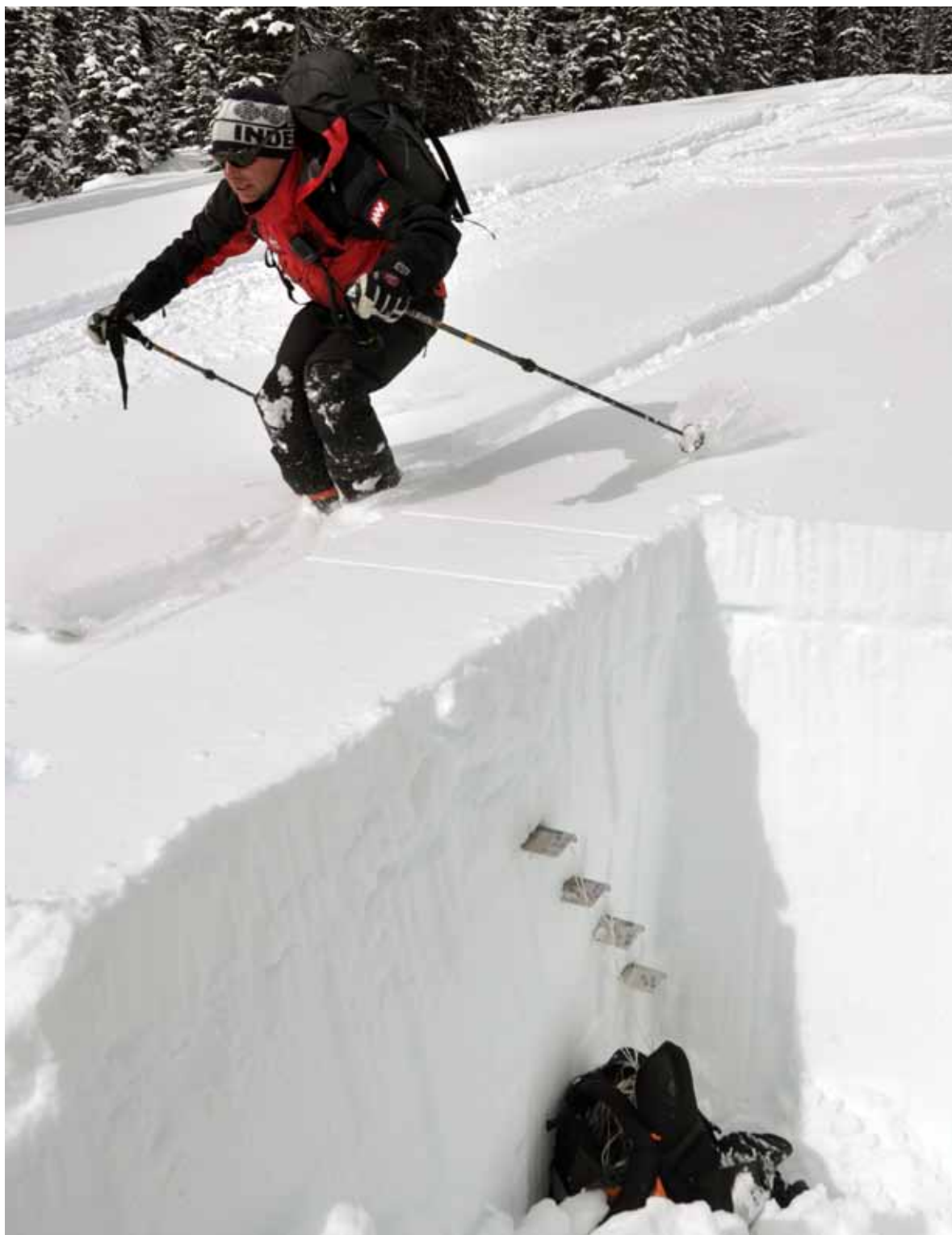
FIG. 1: MIKE WHEATER LOADING THE SNOW SURFACE ABOVE THE SENSORS. THE SENSORS ARE MOUNTED TO LONG ALUMINUM SHEETS THAT ARE INSERTED INTO THE SIDE OF THE PROFILE. THE DATA LOGGER IS IN THE BLACK BAG.
