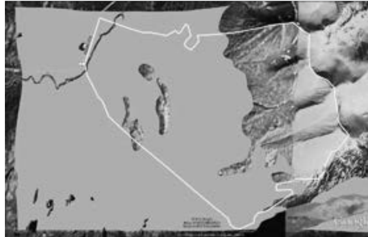
FIG. 2: IN THE ABSENCE OF HIGH RESOLUTION IMAGERY, VEGETATION OVERLAYS CAN BE USED TO SUPPLEMENT THE LOW-RESOLUTION IMAGERY TO GIVE A BETTER INDICATION OF FOREST COVER. THIS PARTICULAR EXAMPLE SHOWS FORESTED AREAS IN GREY.
