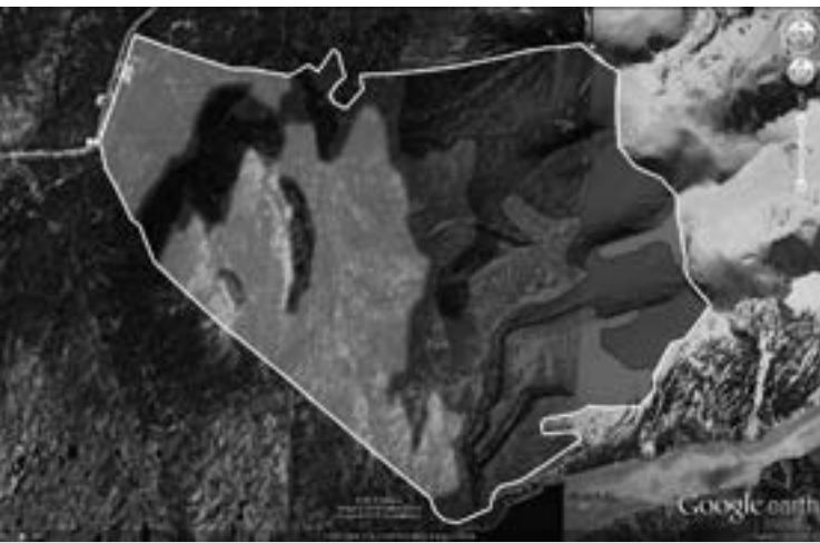
FIG. 4: FINAL ATES OVERLAY FOR THE TUTSHI CHUTES AREA IN THE YUKON SHOWING CLASS 1 "SIMPLE" TERRAIN SHADED IN LIGHT GREY, CLASS 2 "CHALLENGING" TERRAIN SHADED IN DARKER GREY, AND CLASS 3 "COMPLEX" TERRAIN SHADED THE DARKEST. THE ATES POLYGON OVERLAP, EXPRESSING UNCERTAINTY AND ERROR, CAN ALSO BE SEEN.
