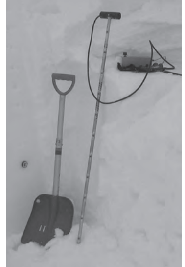
Above: The temperature profile probe sitting next to a shovel for size comparison. Below: The data logger. The LCD screen shows the temperature profile function.
