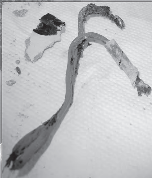
The photo of the thawed out cap/fuse assembly clearly shows the end of the blasting caps where they are crimped to the fuses, as well as at least 4 cm (1.5 inches) of the cardboard tube detonator wells. This shows the detonators were properly installed.
