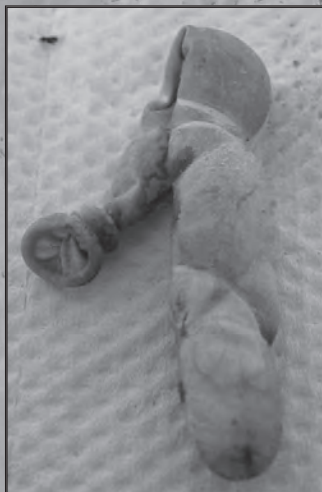
The balloon that contains the sensitizing compound for the bulk of the cast shot was found about 10 metres (30 feet) from the blast crater. Notice the striations left from the rubber band.
