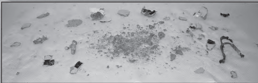
Material retrieved from the misfire site. Notice the PETN balloon in the left center of the photo.
