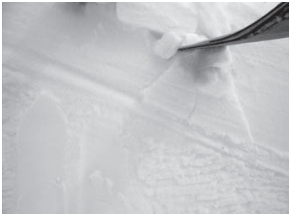
Photo 3: This is an example of excavated tracks from a ski cut where the skier did initiate a weak layer fracture beneath their skis, but the fracture didn't propagate to release an avalanche. In this case the propagation propensity would be low, even though triggering was easy.
