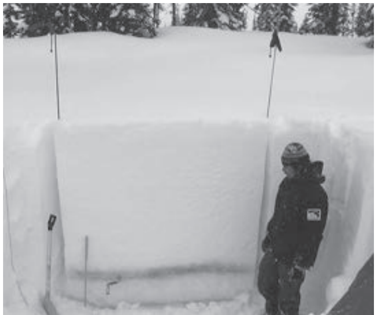
Photo 2: The slab we tested here was over 150 cm thick, and results from testing on this flat terrain were almost perfectly reproducible on nearby slopes. The PST works with slabs of any thickness, but columns like these can take 30-45 minutes to prepare. The three metre thick ones take hours.
