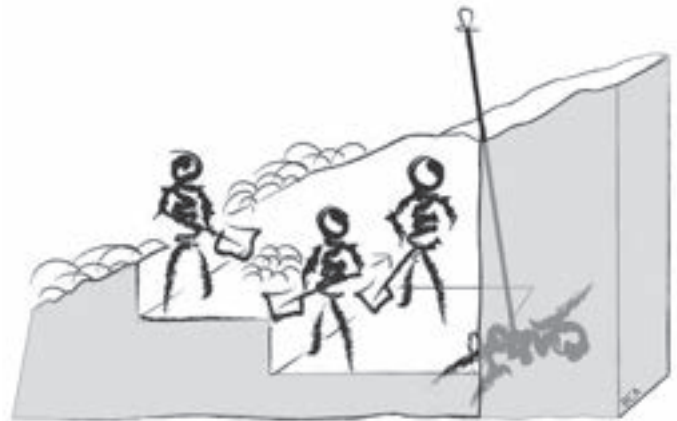
Figure 4. In burials deeper than two meters, it can be difficult to clear snow from the hole. Instead, it should be lifted to the next terrace, where it is removed by a secondary shoveler.
