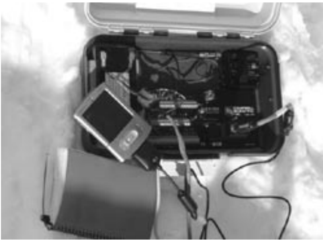
Figure 3: Recording setup. Note CR1000 datalogger, large 12 V lead acid battery for the datalogger on the left under the Palm Pilot, and 9 V battery bank for the supply voltage to the penetrometer tip.
