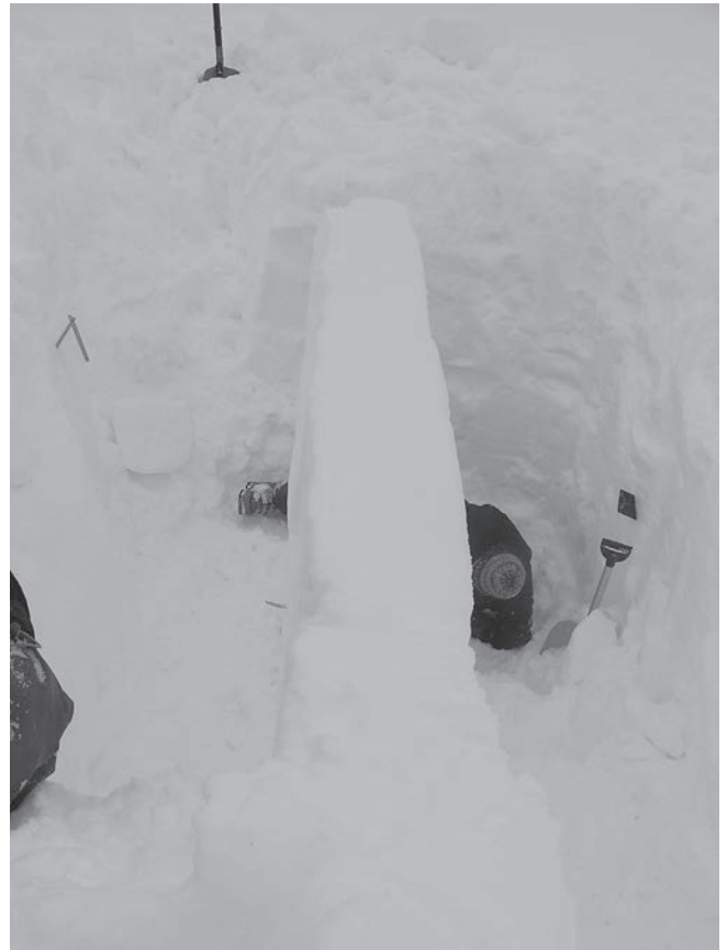
Looking down at the “big beam” on Cheops Bench. The beam was 30 cm wide, 285 cm long, and excavated to a depth of about 2 m. The 060126 surface hoar layer was 170 cm below the surface. I’m deep in the trenches taking a close look at the weak layer in the area that the saw passed through. The collapse ran toward the camera.
