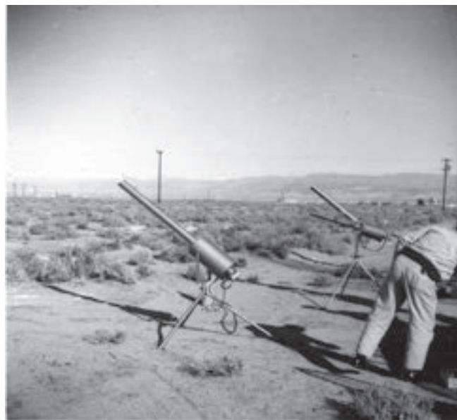
A "Fireball" baseball-pitching machine in the background and a prototype Avalauncher in the foreground. Photo taken in late 1971 by Monty Atwater.
