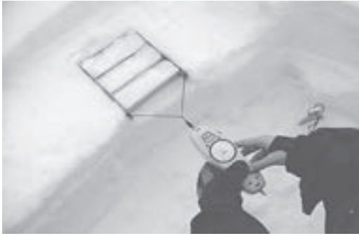
Figure 1 – Shear Frame Test
