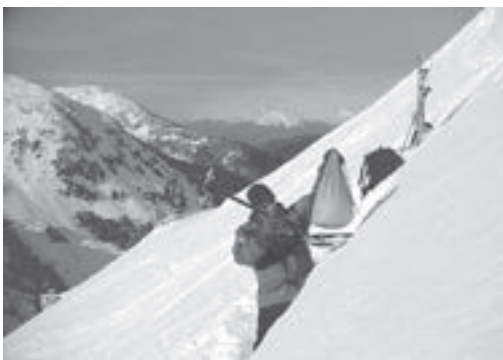
Figure 2 – Conducting a Stuffblock Test at Eaglecrest
