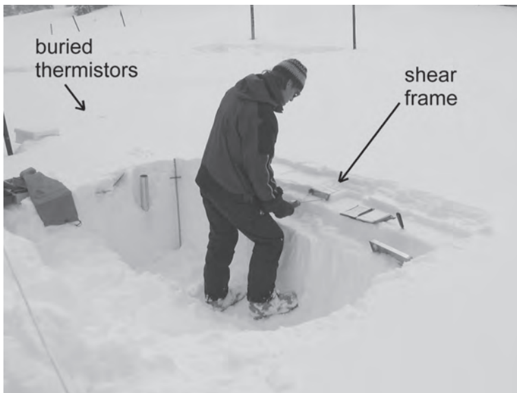
Fig. 3. Photograph of operator performing a shear frame test on a layer of facets on a crust. The bottom of frame is placed a few millimetres above the facet-crust interface and pulled to fracture within a second. The layer being tested was buried 2004-01-15 at Mt. St. Anne.
