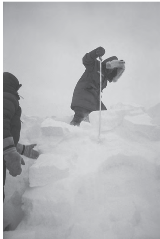
A snowshoe ruschblock test at the Giant Goldmine Tailings Pond in Yellowknife.
