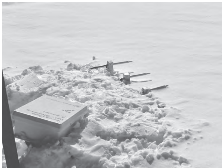
Fig. 2. Photograph showing three vertically oriented pairs of thermistors that were placed in wet snow before dry snow fell. Only the top thermistor of each pair is visible above the dry snow. The thermistors are connected to a datalogger in the white box that reads each temperature every two minutes and records the average temperature of each thermistor every hour.
