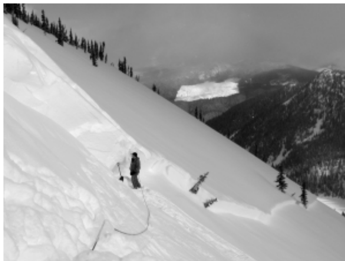
Fig. 1. Photo of observer at crown of a natural dry slab avalanche that slid on a layer of faceted crystals within a layered melt-freeze crust.
