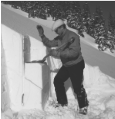
Figure 10. For this Deep Tap Test, the upper column has been removed to test a deep weak layer. Along the sidewall, the deep weak layer has been notched 5 cm with a straight snow saw. The tapping is the same as for a compression test.
